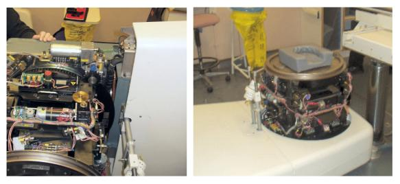
The head assembly, inside which is the x-ray target. This, at least, is one complex item which we will not need.
