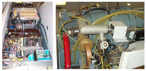
Details of the accelerator: The gun and magnetron drive circuits on the left and details of the gun assembly on the right.
