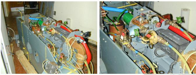
Even though the interconnections between the basic components in the linac's radiofrequency system are straightforward, we all know that it is easier to take apart than to put together again. Reverse-engineering a complex bit of kit can be full of unexpected surprises. So detailed, very detailed and very, very detailed pictures are always a good idea. Here is a selection showing the magnetron, the isolator and the output waveguide.
