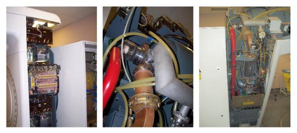
Details of the accelerator: The focus supplies on the left, the gun, mode transformer and vacuum pump in the middle and the radiofrequency generator on the right.
