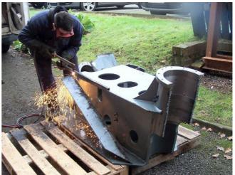
Flame-cutting the frame of the linac....all that's needed is to do it along a straight line and then to smooth the edges with a grinder. An excellent professional such as Rod makes it look, well very easy!
